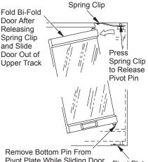
Pivot Plate While Sliding Door Pivot Plate Out of the Upper Track
